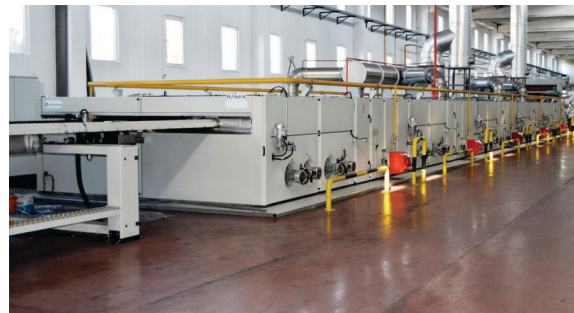
Fig. 13. A stenter machine with economizer installed
