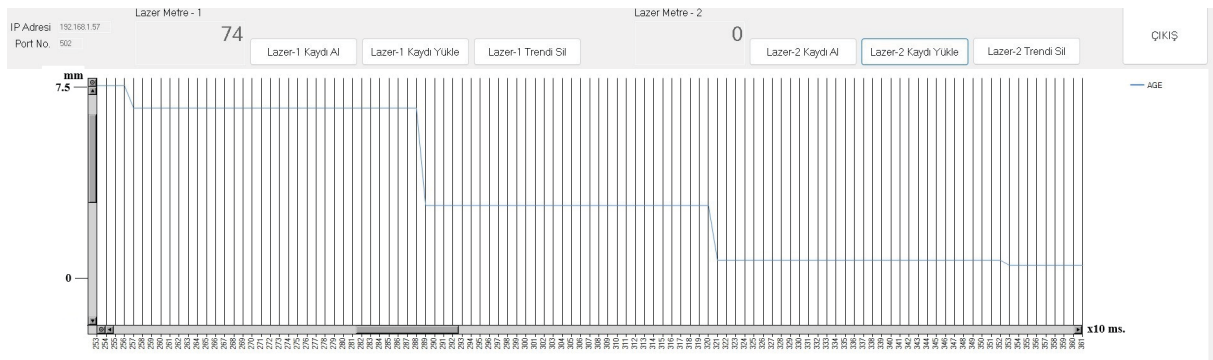
Fig.10 Triple PZT crystal test specimen's Experimental linear displacement-time result at 220 V Voltage
