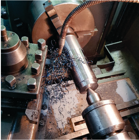
Fig. 1. Experimental setup (minor cutting edge angle of \kappa_1 = 25^\circ is achieved by rotating the tool post)
