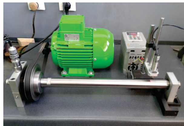
Fig. 2. Appearance of the bearing test rig
