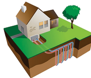
Fig. 3. Vertical ground heat exchanger [6]
