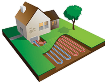
Fig. 2. Horizontal ground heat exchanger [6]
